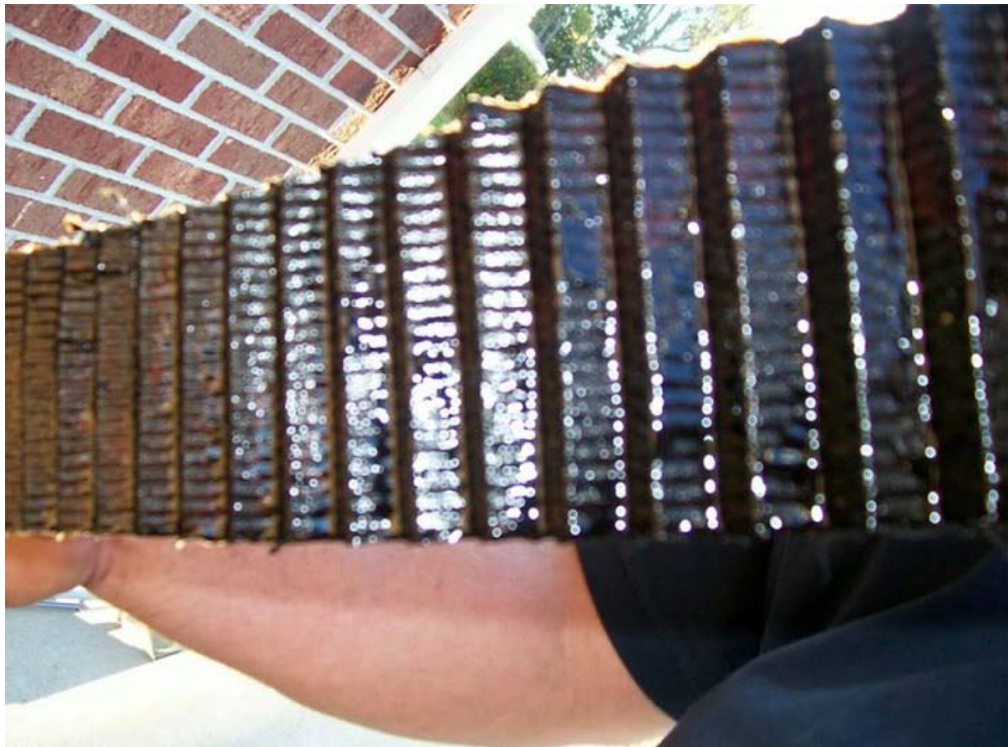
Here is the filter media from the AATG filter used during the cleaning phase. It's got a lot of pasty, syrup looking black goo in it.
