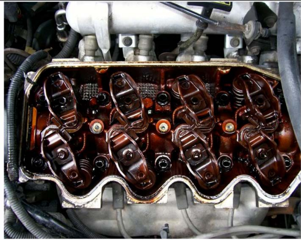
Original photo of valve train, before Auto-RX treatment. Note that this valve train is pretty clean to begin with. Some slight brown varnish coating, but no sludge..
